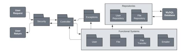
The above graphic displays the components of the back-end of the application. A standard user request will be passed through security where the controller will then send the request to the correct functional system. The functional system then interacts with the corresponding repository in the database. The response is passed back to the
